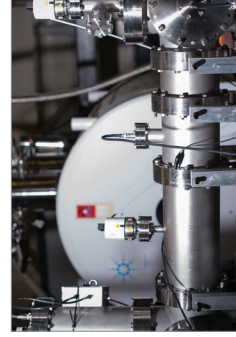
TAMUTRAP (2016) Purifies and confines short-lived ions for precision decay experiments and as a general decay station.
