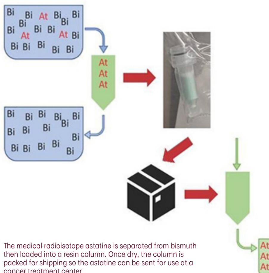
The medical radioisotope astatine is separated from bismuth then loaded into a resin column. Once dry, the column is packed for shipping so the astatine can be sent for use at a cancer treatment center.
