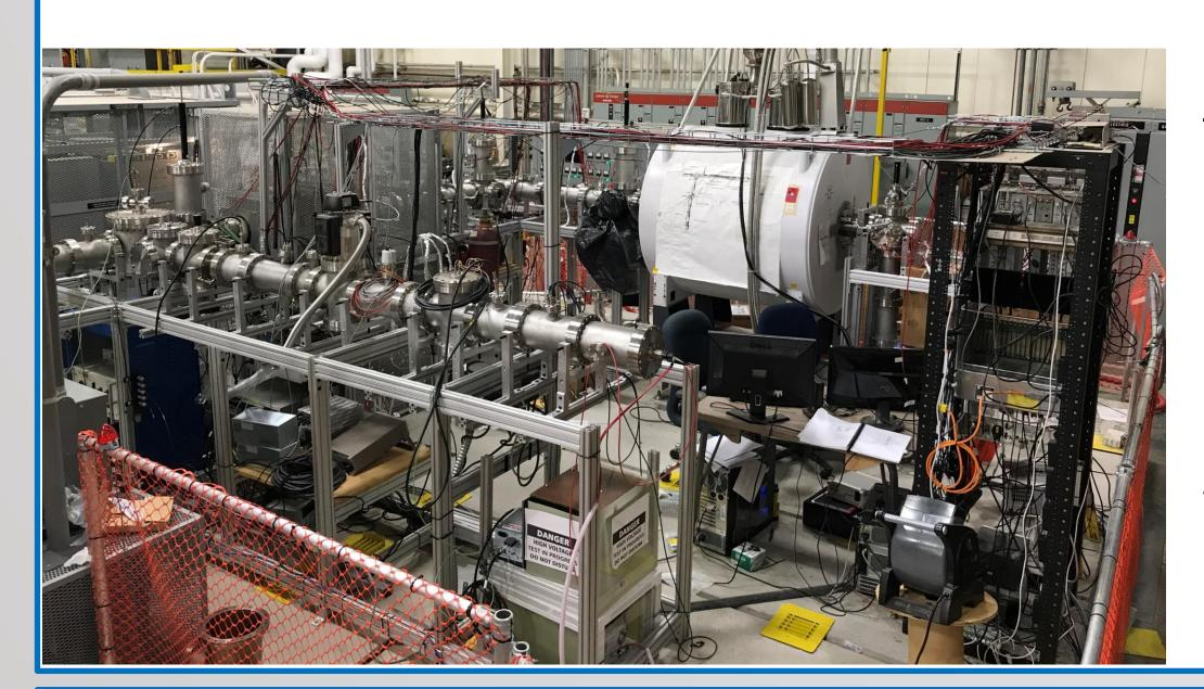
The beamline is a complex set of deflectors, lenses, and steerers in order to control the path the ion takes while traveling to the Penning trap.
