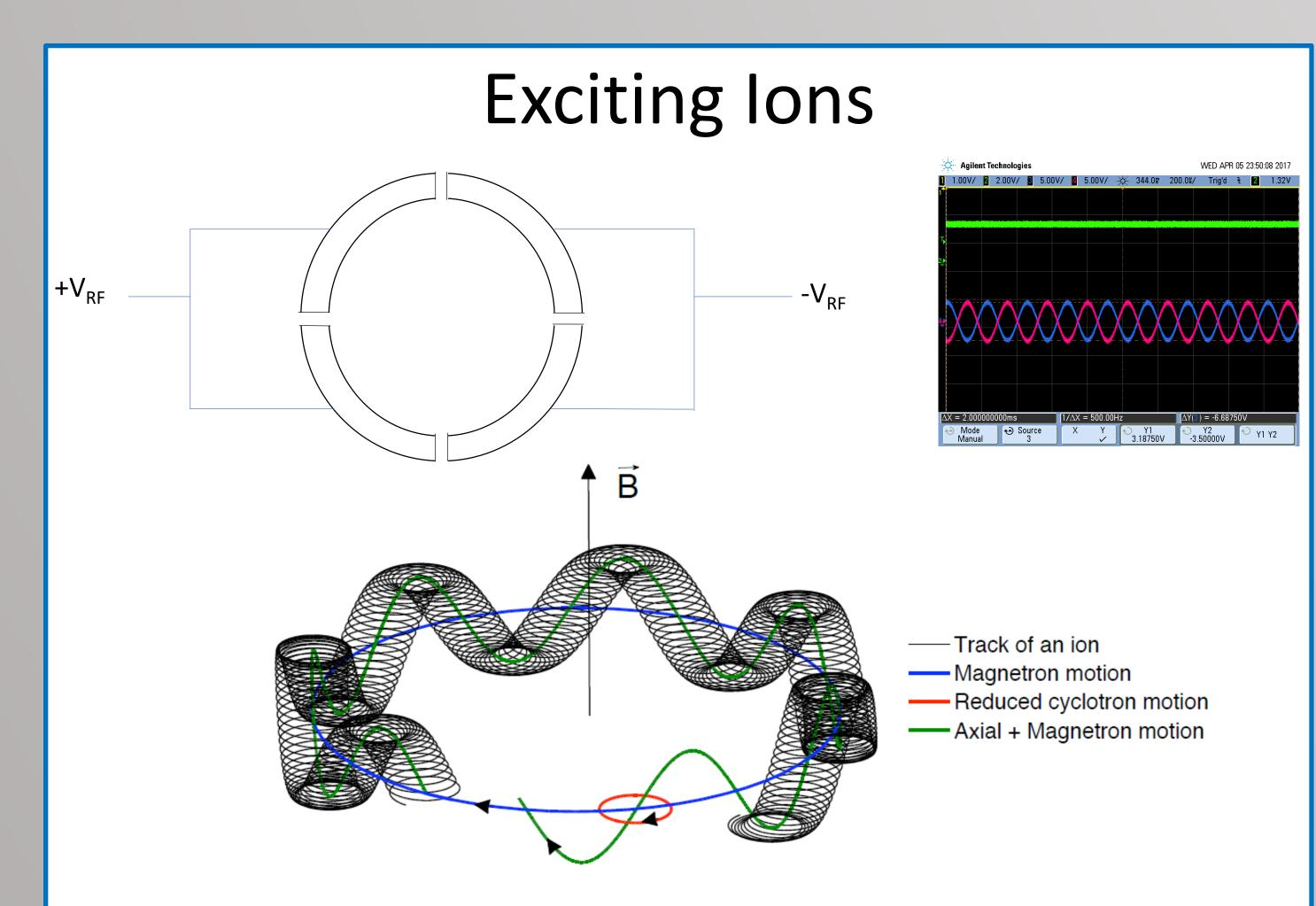
The ions are excited by alternating radiofrequency voltages on the segmented center ring electrode. At resonance, these equalmagnitude, but 180° out-of-phase, sinusoidal voltages cause the ions to rotate in different motions. Once the ions become excited, they are shot through the end of the trap to a detector.
