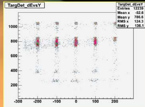
A diagnostic run using a test nucleus ( $^{13}\text{N}$ ) was performed in late July 2004. The preliminary data shown was taken with the polarity reversed on quadrupoles 4 and 5 and detector slits 3 and 4 open. This demonstrates an "unbeam" before purification.
