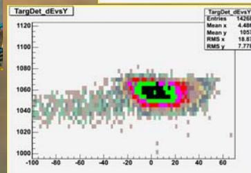
With the polarity of the quadrupoles corrected and the filtration slits closed the beam is focused to an area ~6 mm wide and ~9 mm high.
