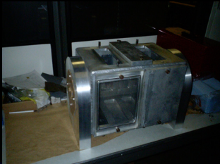
Refurbished and Assembled Beam box
