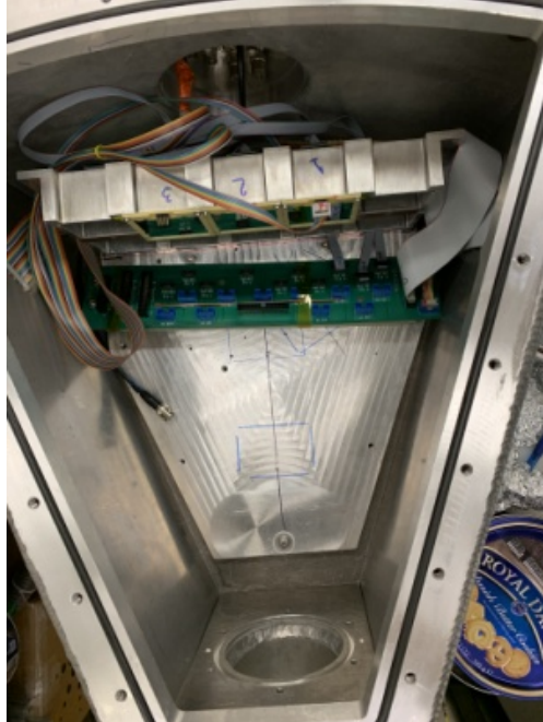
FIG. 1. Picture of the experimental setup. The picture shows the scattering chamber and the three Si-CsI(Tl) telescopes (labeled as 1, 2, 3) at the end of the gas volume. A PCB board used for the signals read out is also visible.
