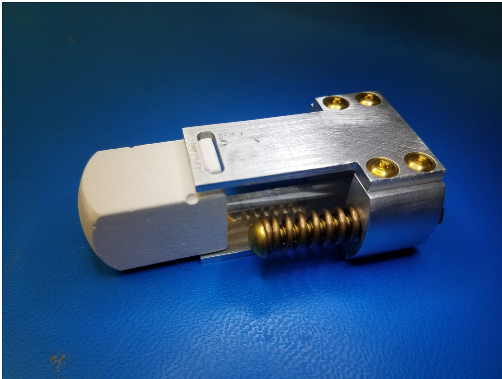
FIG. 1. Prototype primary optical lens in non-magnetic fixturing.
