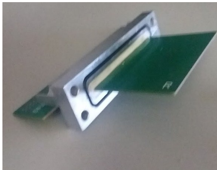
FIG. 3. Feedthrough after potting.
