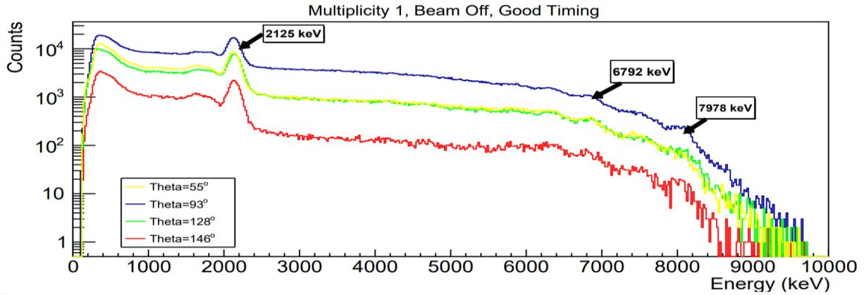
**Fig. 2.** Gamma spectra measured in the four sections of the TexCAAM array during beam off.
