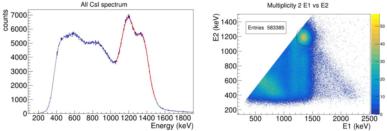
**Fig. 3.** Left panel: Spectrum of the  $^{60}\text{Co}$  source. The red line shows the result of the fit with two Gaussians and a linear background. Right panel:  $^{60}\text{Co}$  source, multiplicity two events, E1 vs E2. A two-dimensional gate is plotted around the spot of 1173 keV and 1332 keV gamma ray coincidences.
