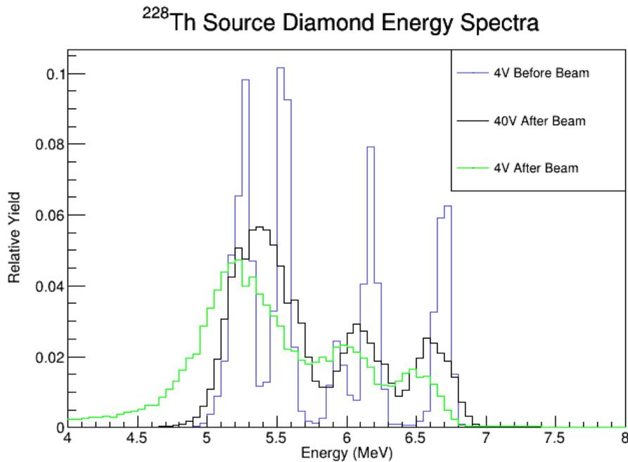
**Fig. 2.** <sup>228</sup>Th alpha spectra in Diamond-DADL telescope configuration. Black is the <sup>228</sup>Th spectra with the diamond biased to +40 V while in green it is biased at +4 V. In blue is the same detector biased at +4 V before the experiment.
