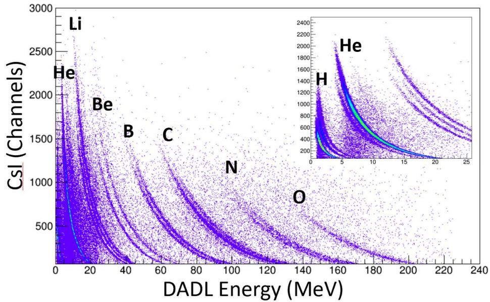
**Fig. 3.** DADL energy (MeV) as a function of CsI (Channels) for a single detector telescope in ring D of FAUST of reaction products from 17 MeV/u  $^{20}\text{Ne}$  on  $^{12}\text{C}$ . The inset shows a zoomed in view of H and He isotopes.
