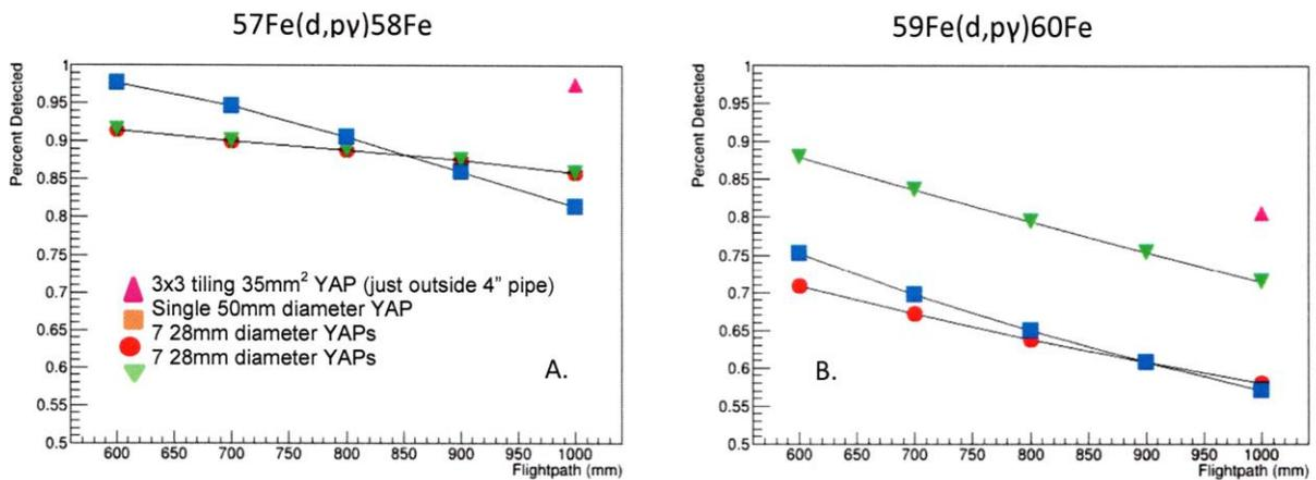
**Fig. 2.** Percent of residues collected given the geometry of the YAP:Ce array for the stable beam (A) and the radioactive beam (B) as a function of the distance of the array from the target position.
