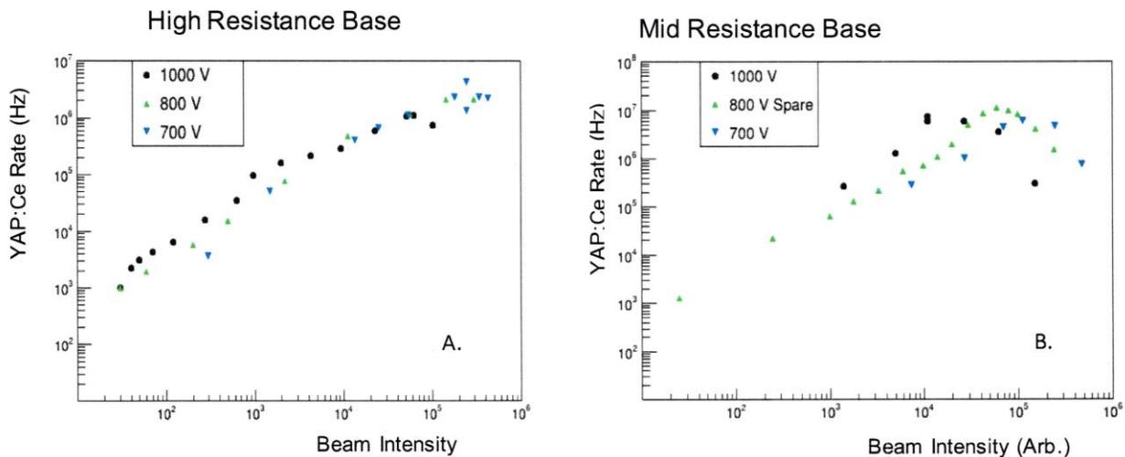
**Fig. 1.** The resulting YAP:Ce saturation rate as a function of the beam rate measured by a plastic scintillator for both the high (A) and mid (B) resistance bases at various voltages. The HR base achieved a maximum  $1.2\text{E}6$  pps at 700 V while the MR base achieves  $1.0\text{E}7$  pps around 800 V.
