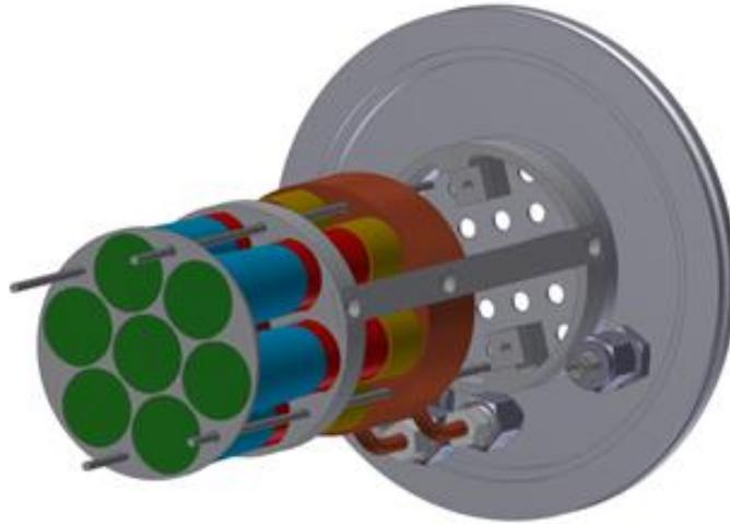
**Fig. 3.** CAD drawing of the YAP:Ce array. The green circles represent the YAP:Ce crystals, the blue cylinders are UVT light guides, the red cylinders are the 1924A Hamamatsu PMTs, and the gold pieces are the active bases. The bases are then slotted into an actively-cooled copper block (bronze).
