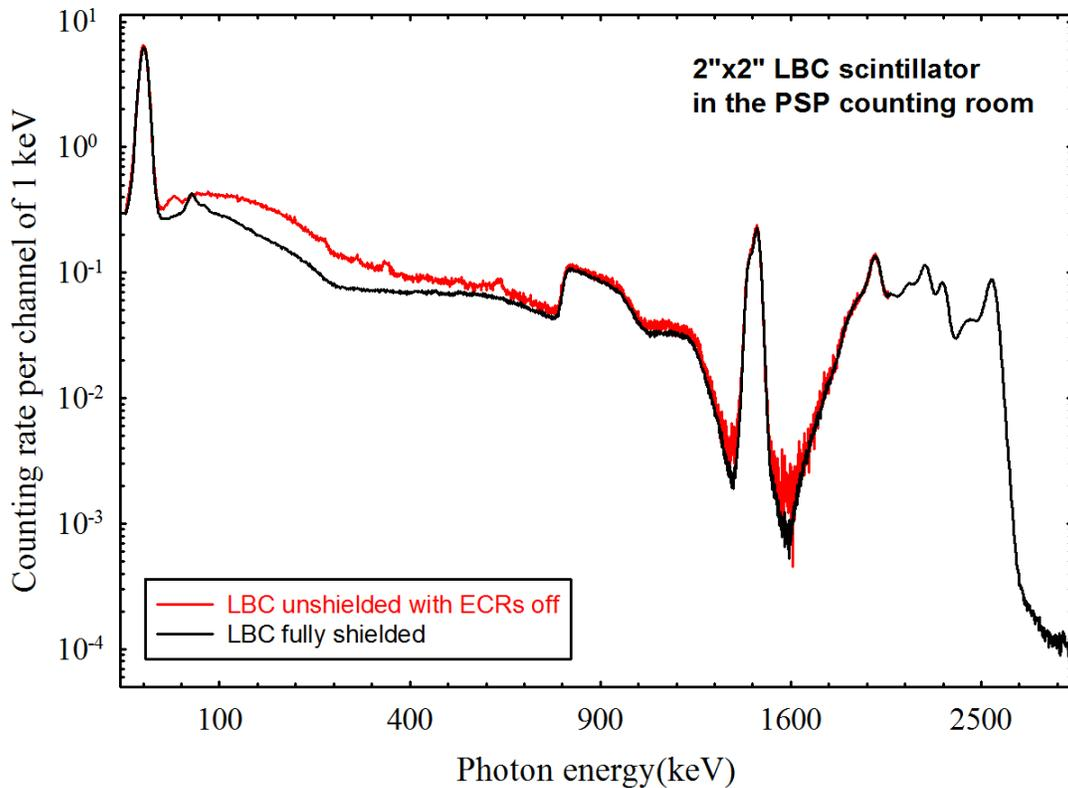
**Fig. 1.** Spectrum of the LBC detector background.
