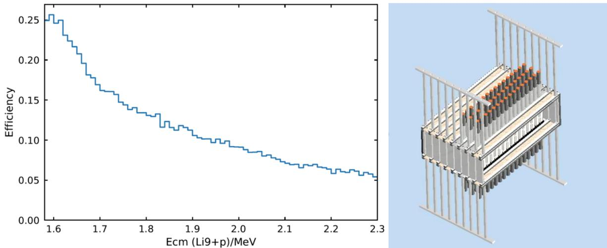
**Fig. 2.** The simulated efficiency of neutrons from  ${}^9\text{Li}(p,n){}^9\text{Be}$  (left) and a CAD drawing of TexNeut in the same configuration that was simulated and that is planned for deployment.
