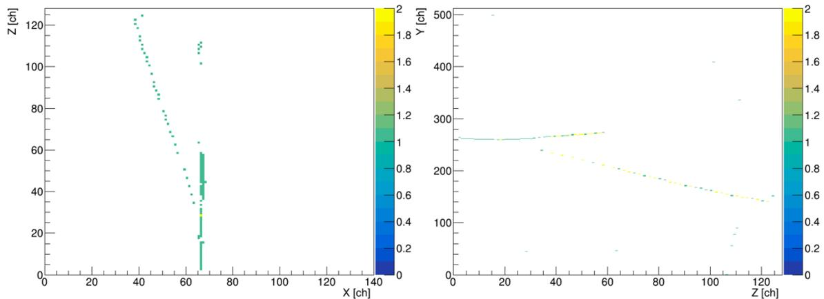
**Fig. 3.** Tracks recorded by the micromegas detectors in TexAT of a suspected  ${}^9\text{Li} + p$  event. This event was selected by gating on the  ${}^9\text{Li}$  beam events and on silicon events within the kinematically allowed energy. These are the X-Z (left) and the Z-Y (right) projections.
