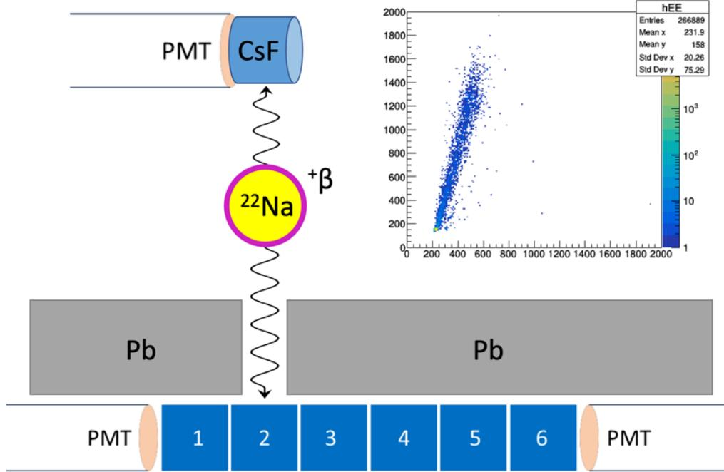
**Fig. 1.** Sketch of the CsF and pseudo-bar placement during the timing characterization experiments. The placement of the stop CsF detector is not shown here. The histogram inset shows the energy spectrum from both PMTs,  $E_{\text{left}}$  vs  $E_{\text{right}}$ , with  $\gamma$ -rays only being exposed to crystal-2 as shown in the diagram. Units in the inset histogram are ADC channel.
