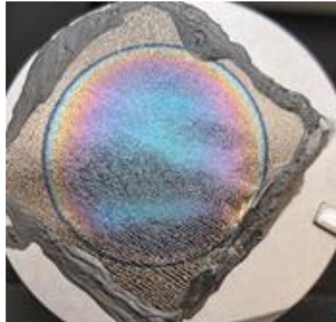
**Fig. 3.** UO<sub>2</sub> target on thin Carbon substrate.
