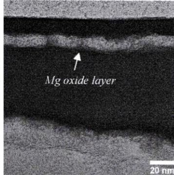
**Fig. 5.** TEM image of a target after heat treatment at 550° and irradiation with  $7.7 \times 10^{16}$  ions/cm<sup>2</sup>
