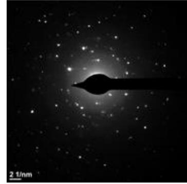
**Fig. 6.** Diffraction pattern of the UO<sub>2</sub> layer after heat treatment at 350°C and irradiation with  $2 \times 10^{16}$  ions/cm<sup>2</sup>.
