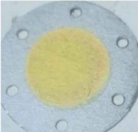
**Fig. 2.** UO<sub>2</sub> target on pure Al substrate.
