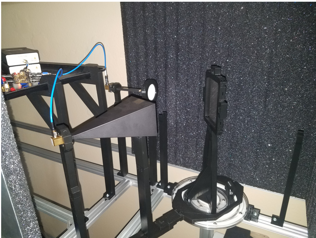
Fig. 1. View into anechoic chamber with calibration plate DUT.
