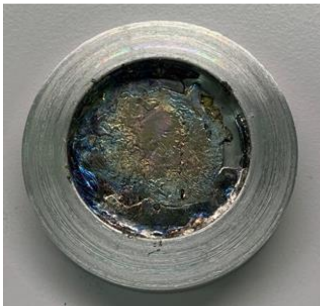
Fig. 2. Bismuth target produced by melting bismuth pellets into the aluminum frame at 310°C and pressed with a heated stainless-steel weight with aluminum foil in between the weight and melted bismuth. The weight and foil were removed while the target was still hot, to prevent adhesion to the surface. The bismuth did not spread fully over the surface, and a colorful bismuth oxide crystalline layer formed on the surface. The total mass of bismuth is 2.649 g, with an average thickness of 210 microns. This target was not used for irradiation.
