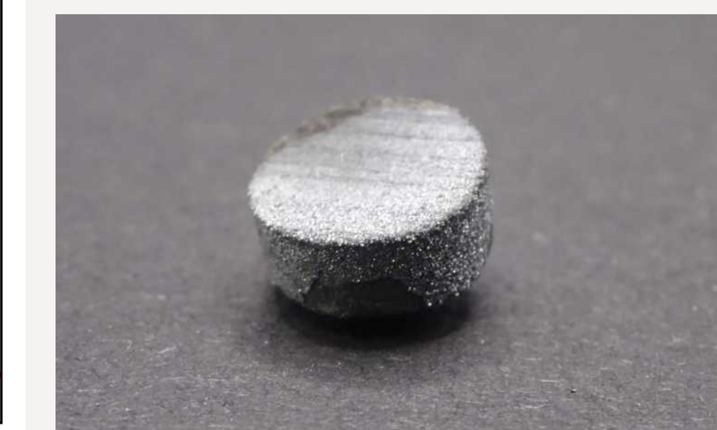
Figure 14: Ti crystals on graphite susceptor
