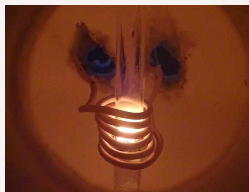
Figure 7: Susceptor at 1200°C
