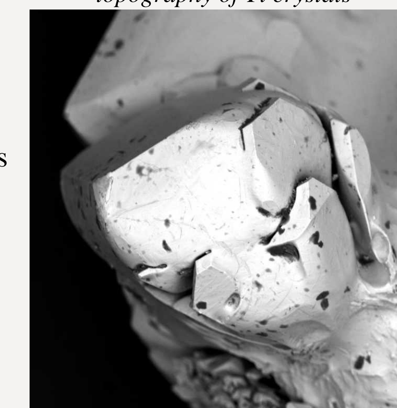
Figure 11: Enlarged SEM view of Ti crystal growth
