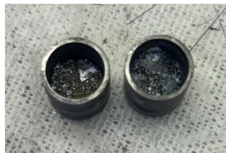
Figure 7: Combined \text{TiO}_2 , Mg metal, and \text{MgCl}_2 pellets in crucible before reduction process.
