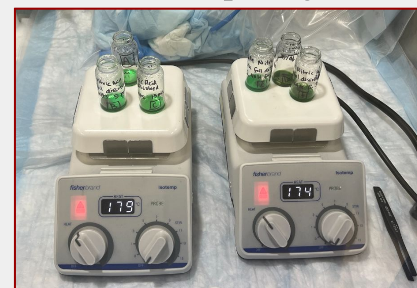
Ni foils dissolved in Nitric Acid
