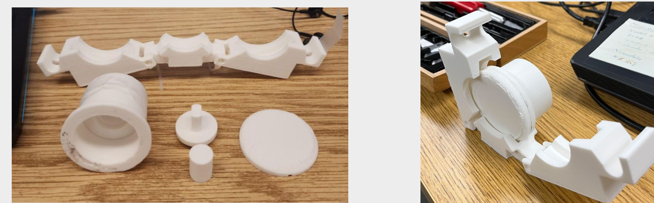
3D Printed Target Chamber Design along with the Single Bolt Flange Design
