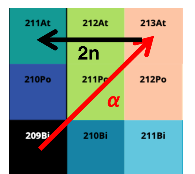
Standard production pathway for ^{211}\text{At} via ^{209}\text{Bi}(\alpha,2n)^{211}\text{At} .
