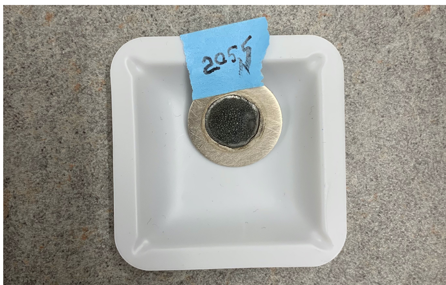
Figure 1. Electroplated ^{\text{nat}}\text{Cr} target. In collaboration with Dr. M. Chernysheva.
