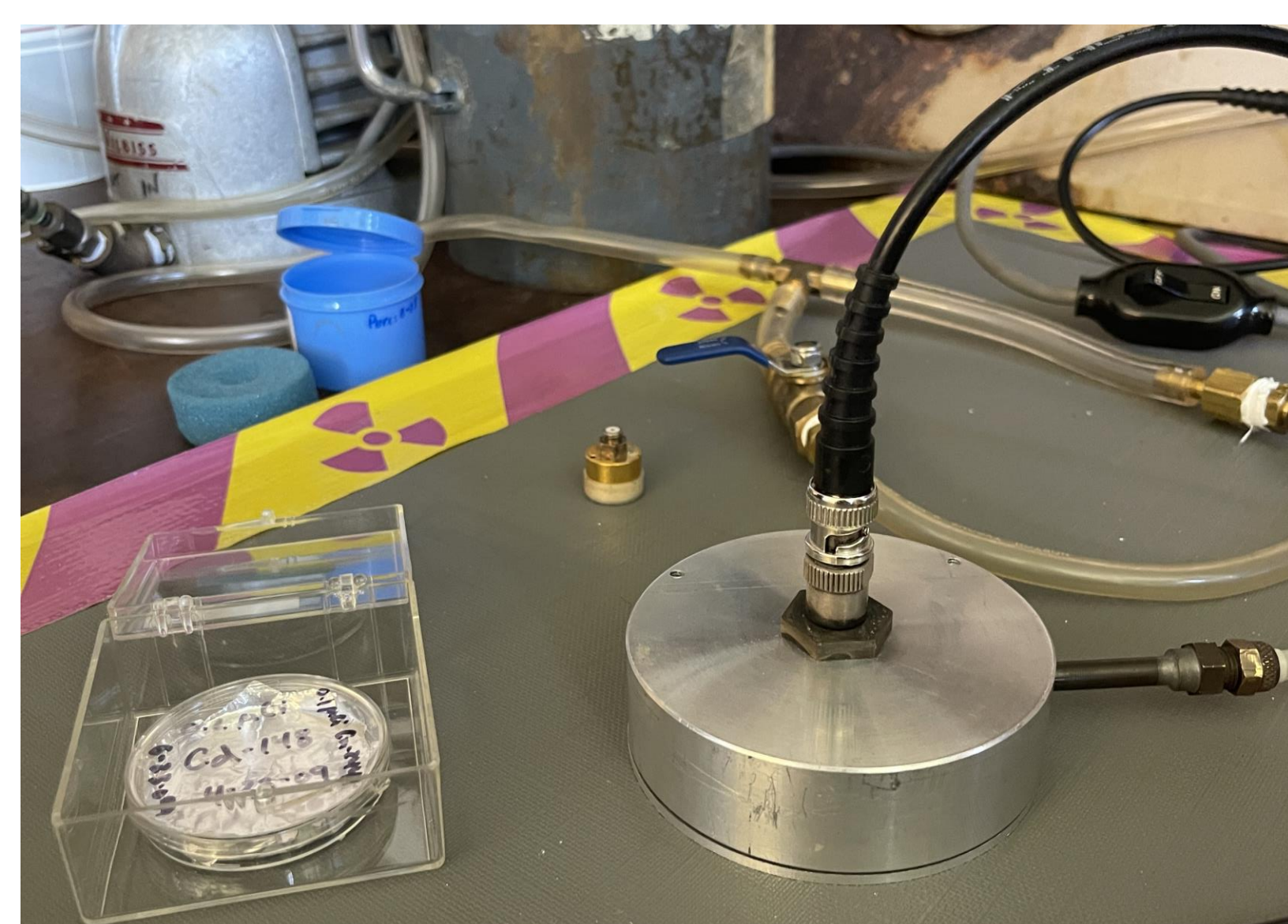
Left picture: Chamber with alpha detector inside and weak alpha source for testing
