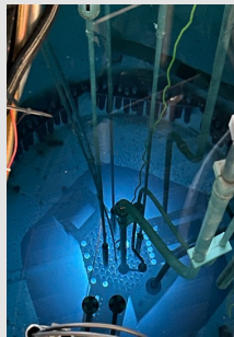
Figure 1 – This figure shows the University of Utah's TRIGA reactor at 90 kW for the enriched irradiation.
