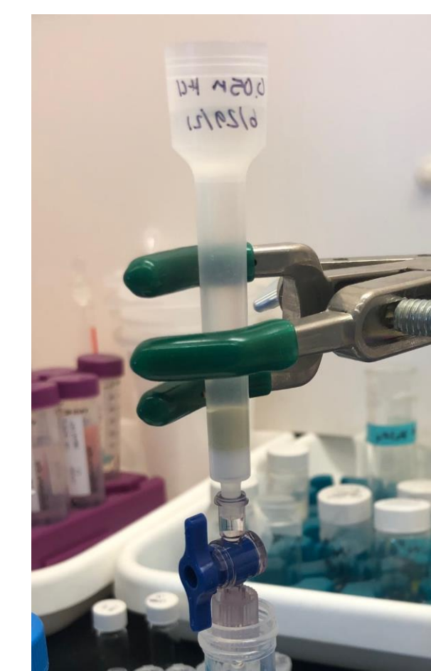
Figure 8. 44 Ti/ 44 Sc generator setup.
