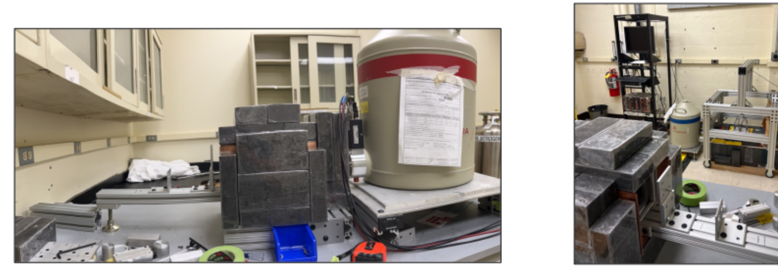
Figure 5: Partially shielded detector (left). Fully shielded detector in background (right).
