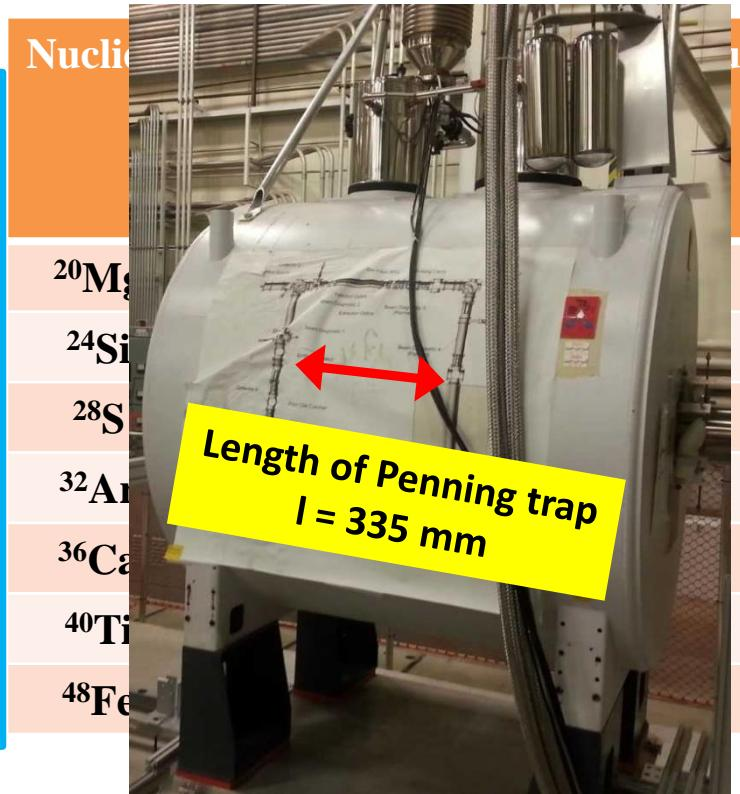
Trap dimensions are also optimized to perform high precision mass measurement.
