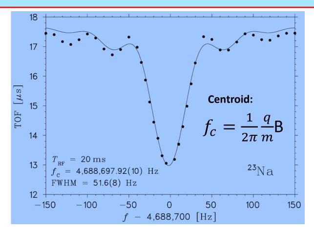
Determine atomic mass from frequency ratio:  $(2\pi f_{c\,ref}) = \frac{q_{ref}B}{m_{ref}}; \ (2\pi f_c) = \frac{qB}{m}; \ m = (m_{ref}) \left(\frac{f_{c\,ref}}{f_c}\right)$
