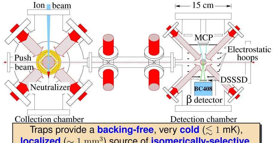
localized ( $\sim 1 \text{ mm}^3$ ) source of isomerically-selective, **short-lived** radioactive atoms
