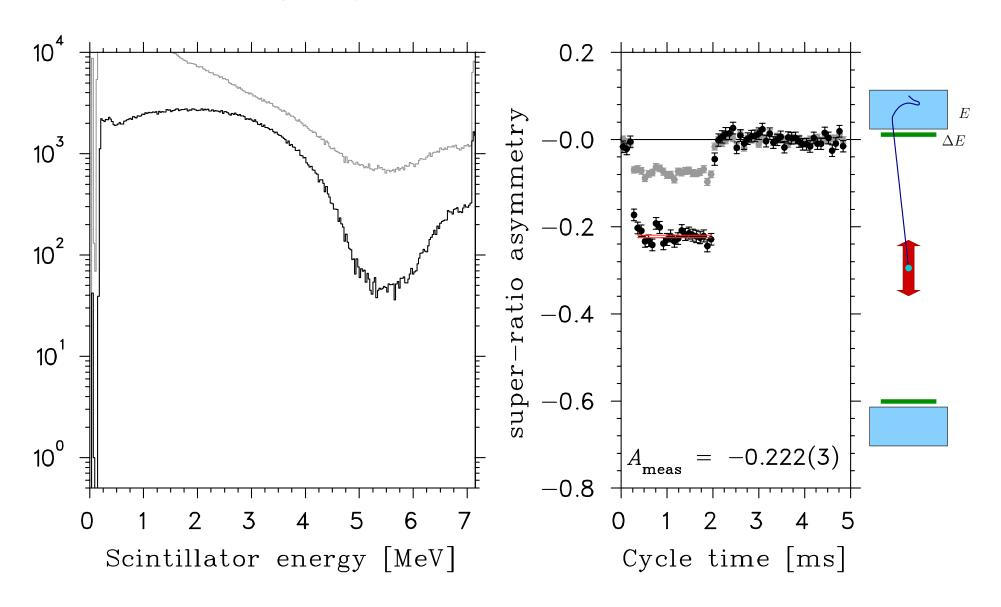
Requiring a shake-off  $e^- \Rightarrow$  decay occurred from trap!
