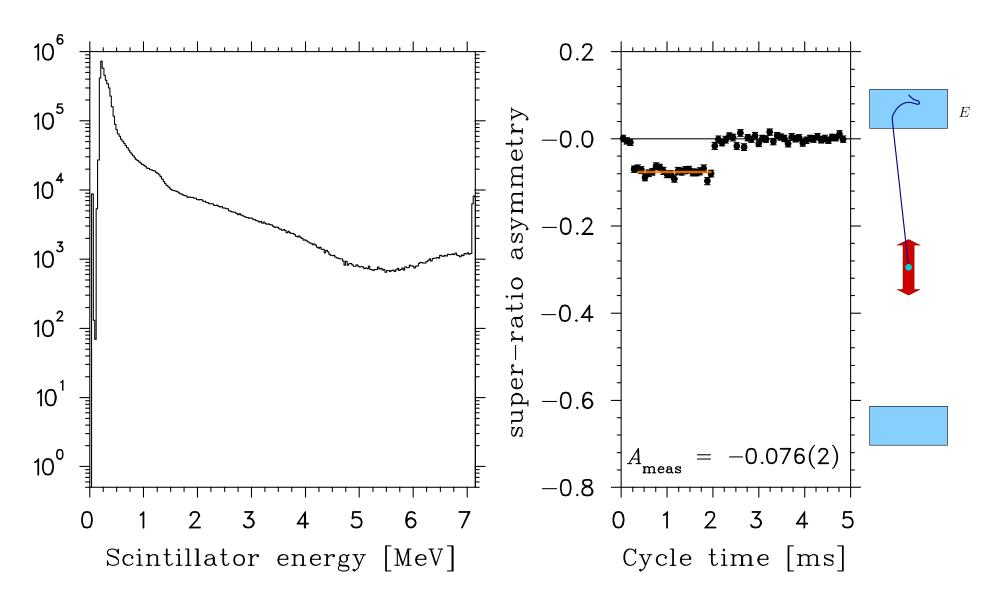
Requiring a  $\Delta E$  coincidence  $\Rightarrow$  remove  $\gamma$ s
