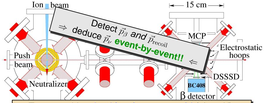
Traps provide a backing-free, very cold ( $\lesssim 1$  mK), localized ( $\sim 1 \text{ mm}^3$ ) source of isomerically-selective, short-lived radioactive atoms
