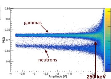
Fig. 5 Previous wavelet transform [2] band separation
