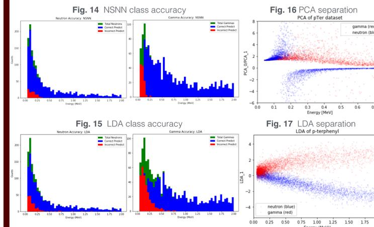
ML is successful above 250 keV. Gamma inaccuracy significantly greater than 50% below 250 keV suggests that the source was too weak to overcome background (Fig 4). Hence, TOF discrimination misidentified background and fission products. Improving a priori identification and reducing background using stronger sources or autoencoding will improve these methods beyond current limitations.
