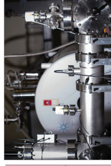
TAMUTRAP (2016) Purifies and confines short-lived ions for precision decay experiments and as a general decay station.
