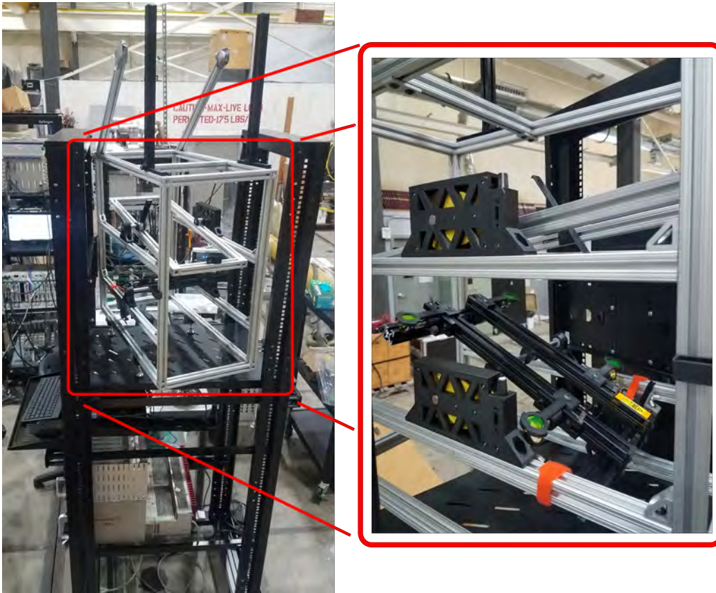
Fig. 1. The receiver cage sitting on its platform in the receiver tower, which houses the support electronics. The inset shows the 3D-printed gearboxes supporting the frames which will mount the beamsplitters and receiver antennas
