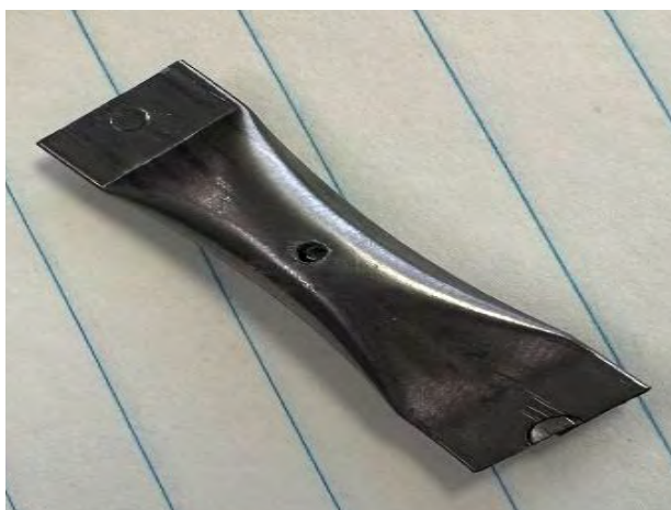
Fig. 1. Tantalum pinhole boat containing a pressed pellet of Sm 2 O 3 and Zr.
