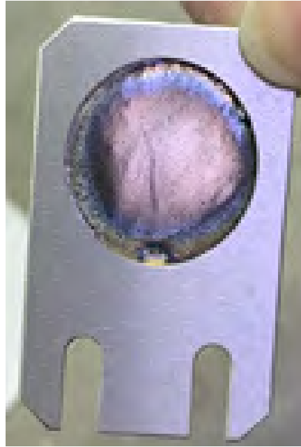
Fig. 2. PVD Sm target with Al backing mounted on a Hyperion frame.
