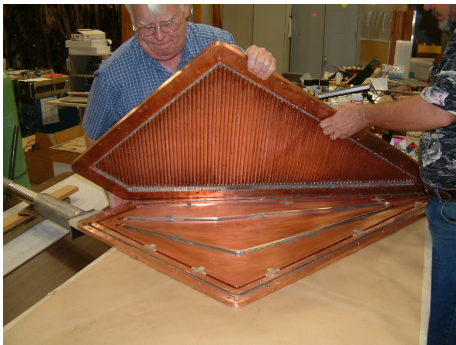
Fig. 1. The K150 cyropanel during its construction.
