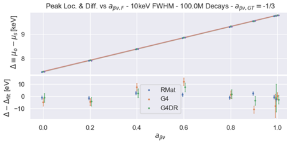
Fig. 2. Separation distance across various a_{\beta\nu} 's. Fluctuation in the fit are eV -scale. The fit serves as a calibration. Given another simulation's \Delta (or experiment), its a_{\beta\nu} can be estimated. RMat and G4 are self-explanatory. G4DR is the G4 with post-imposed 10 keV FWHM detector resolution.
