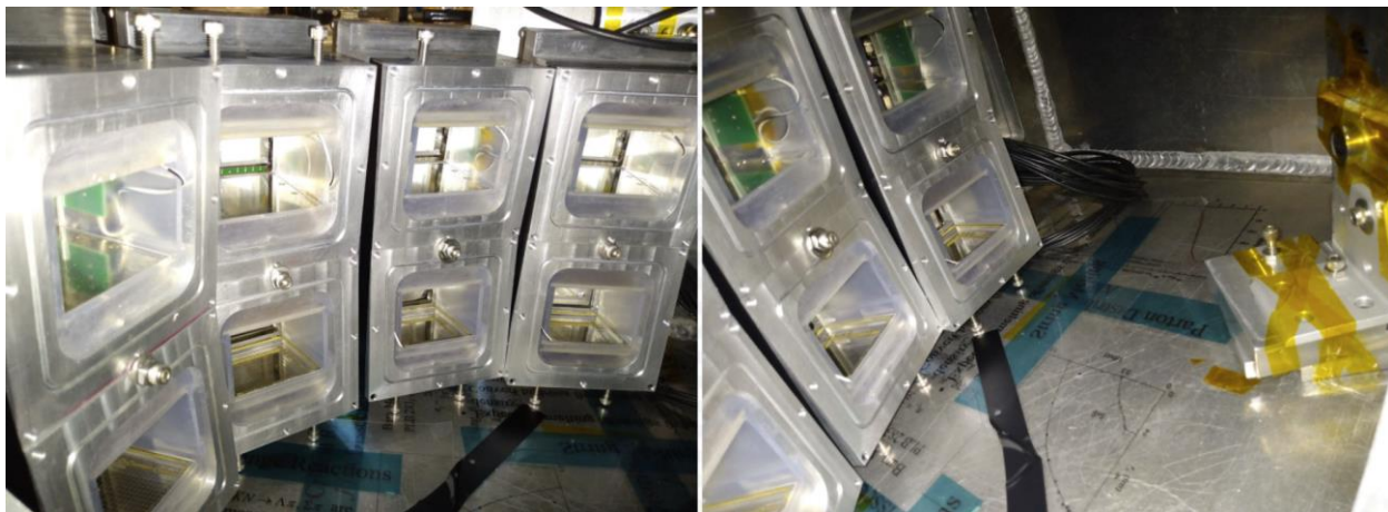
Fig. 5. Setup of detection modules in the vacuum chamber during the calibration runs. The photo on the left figure presents the position of Si modules in the vacuum chamber. The photo on the right side presents the location of the source in front of the detector wall.
