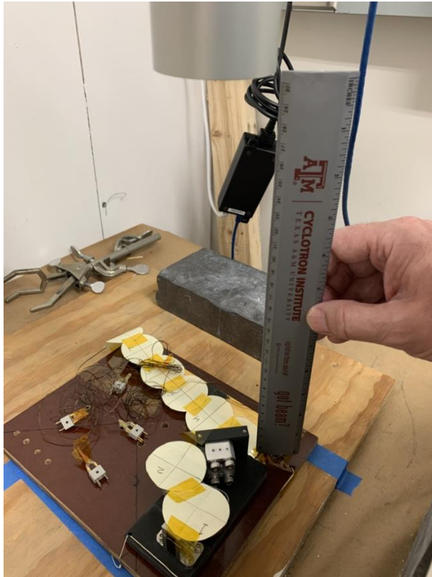
Fig. 1. Devices on a board irradiated by proton beams from the K150 cyclotron.
