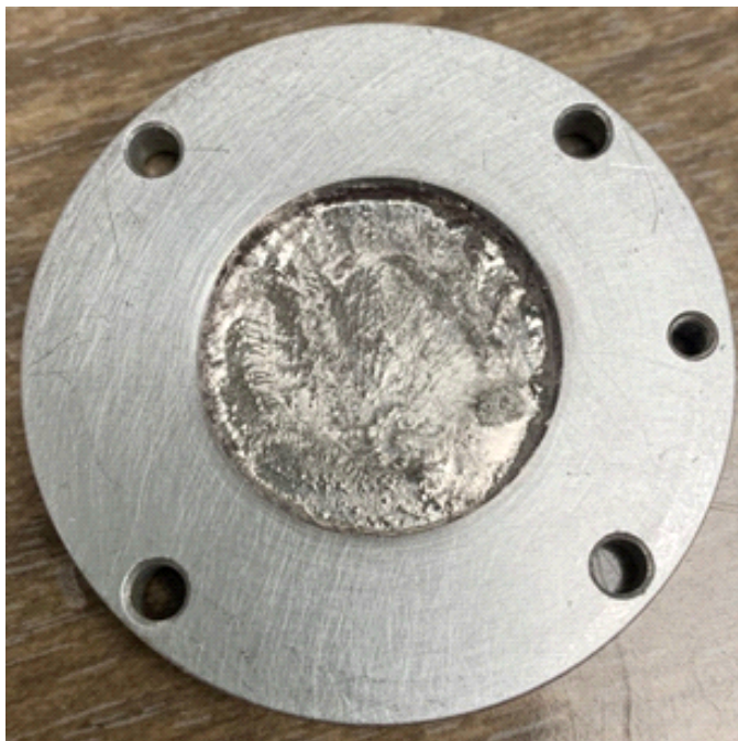
Fig. 3. Bismuth target produced by melting bismuth pellets on a hot plate at 300°C and spreading the bismuth using an ultrasonic soldering iron. The surface is mostly smooth with some ridges and valleys. It has a mass of 0.258 g of bismuth and an average thickness of 66 microns. This target was not used for irradiation.
