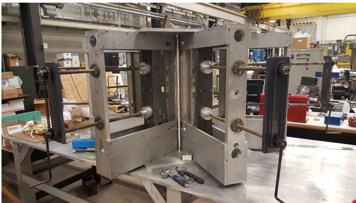
Fig. 1. Fixture used for inserting magnet bars into ECR4 plasma chamber.
