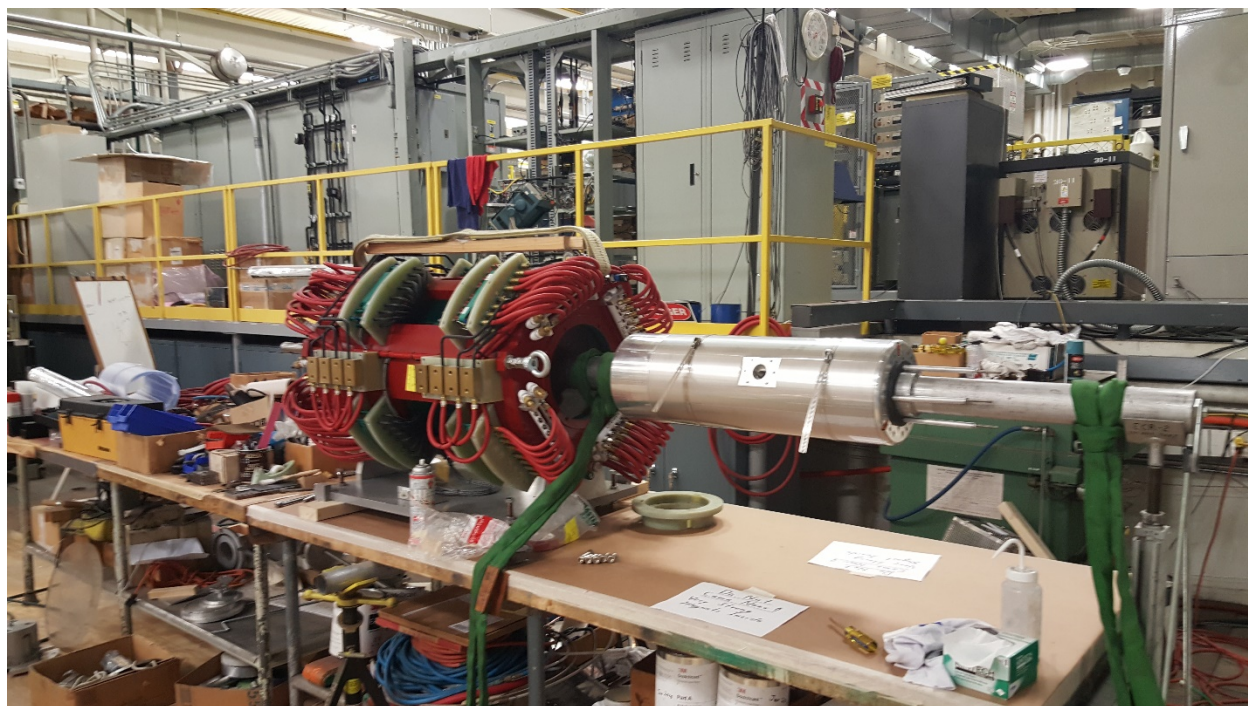
Fig. 2. Plasma-chamber/hexapole being inserted into yoke and coil structure.
