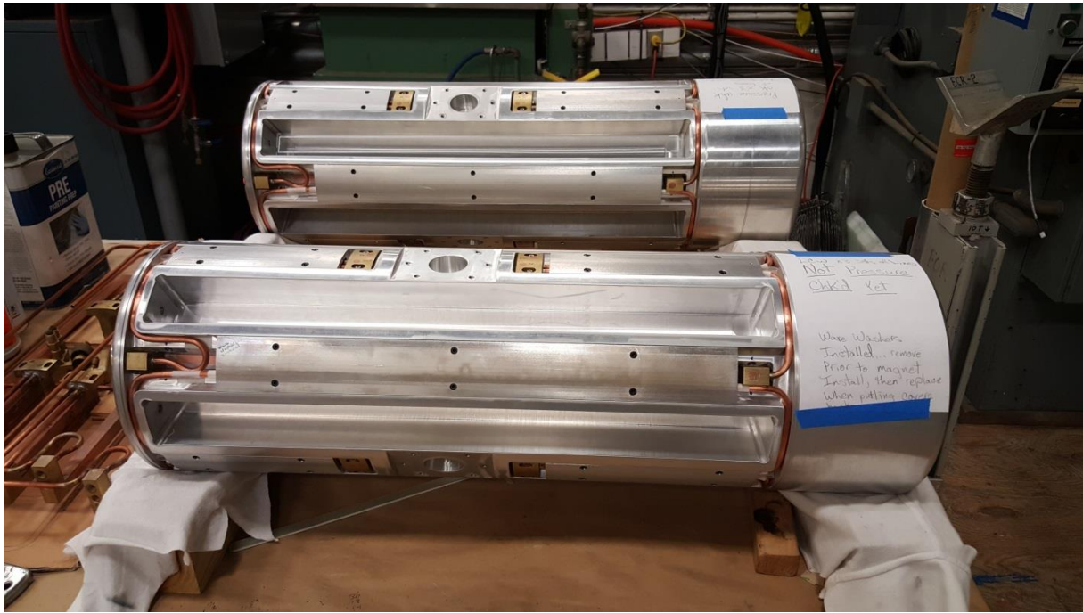
FIG. 1. Plasma chambers for ECR4 and ECR1 with water-cooling channels.
