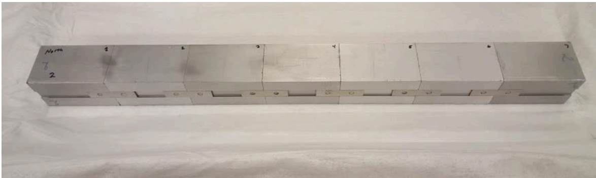
FIG. 2. One of the twelve assembled NdFeB hexapole bars.
