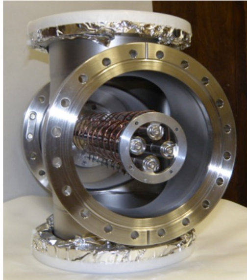
FIG. 1. The 30 cm long DC-drag cooling RFQ assembly.
