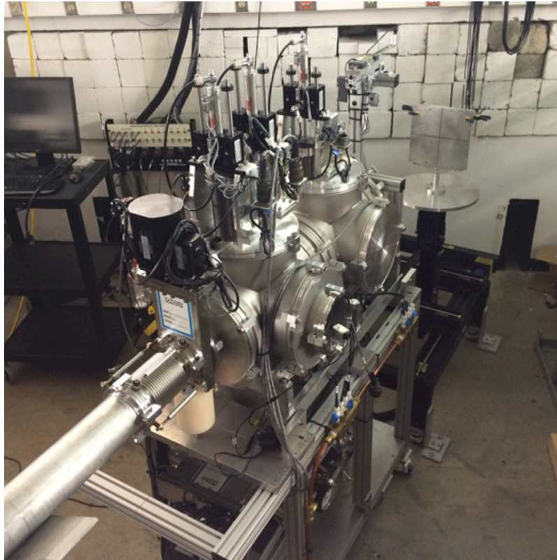
FIG. 1. New Radiation Effects Facility beam line developed for use with the K150 Cyclotron.
