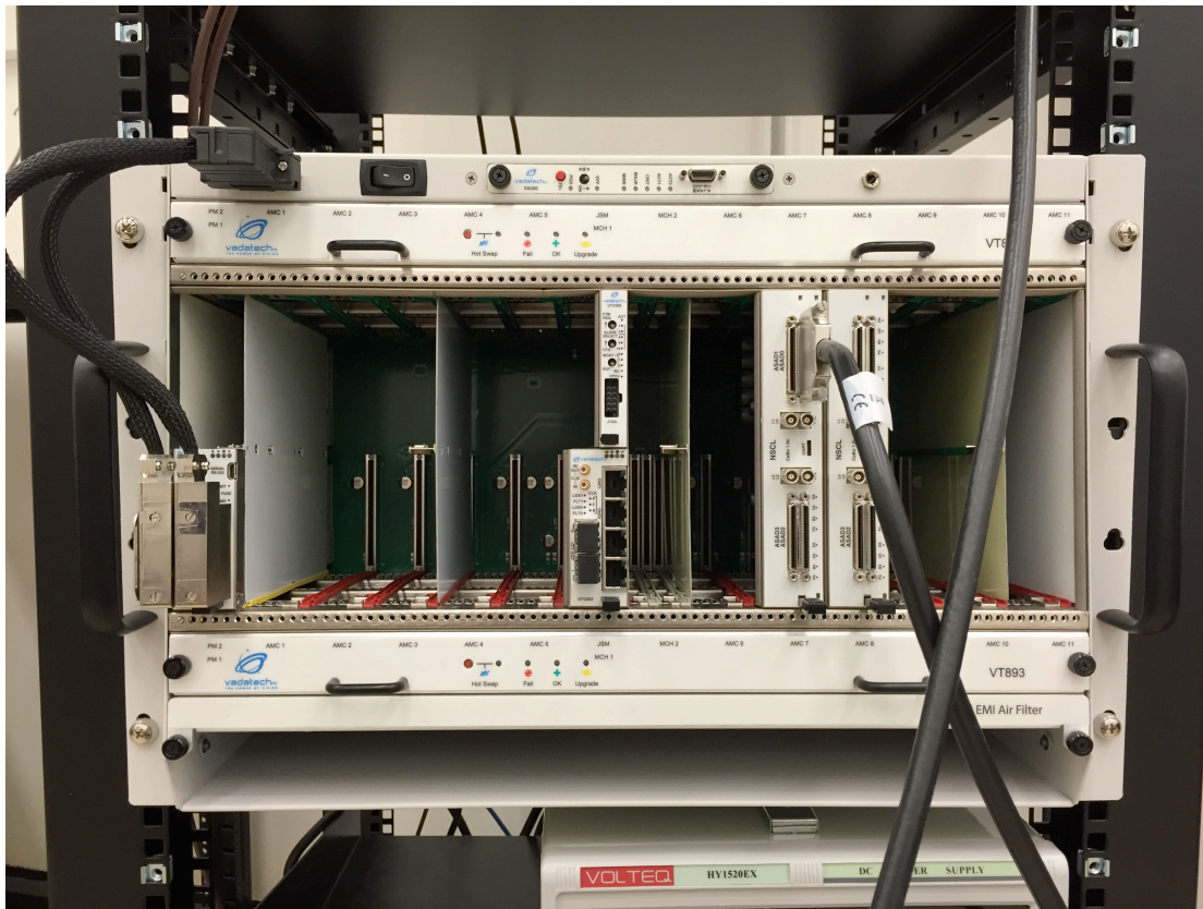
FIG. 2. Image of MicroTCA crate including the two CoBo cards
