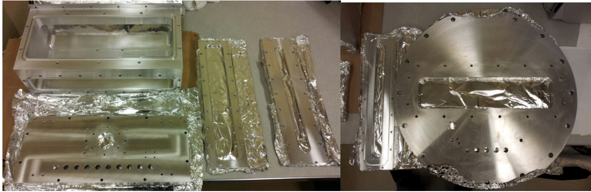
FIG. 2. Duckbill, detector mounting plate, two interchangeable beam windows, beam window transition plate and Duckbill mounting flange with feedthrough holes.
