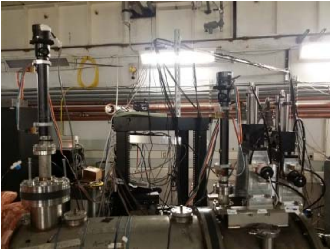
FIG. 1. Two stepper motors and two solenoids on top of the FAUST chamber in cave 2B.
