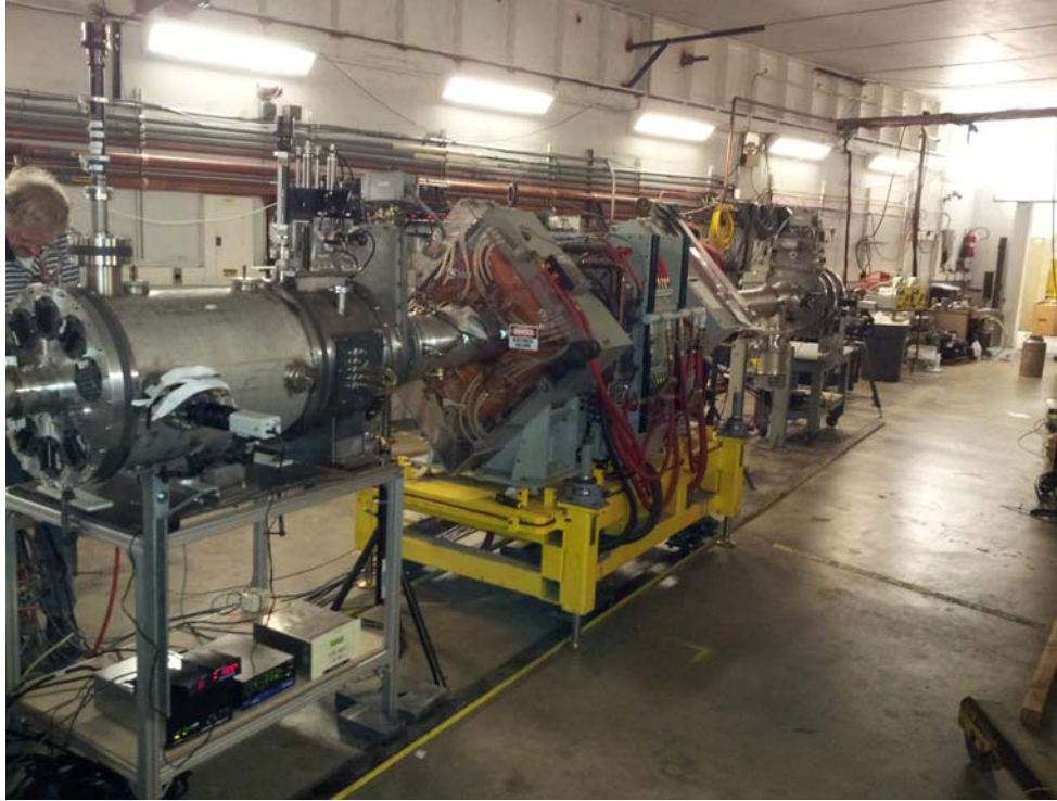
FIG. 2. Actual picture of the FAUST-QTS line assembled and vacuum tight ready to be populated with detectors and cabled to data acquisition electronics. Picture taken in April 2013.
