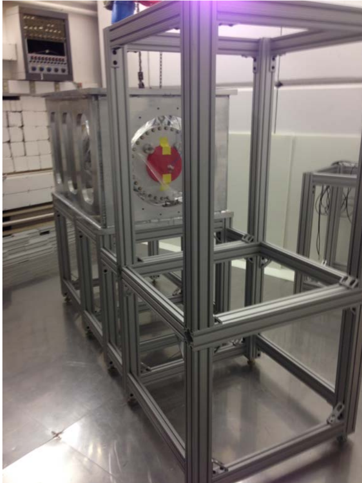
FIG. 5. The support stand with the vacuum box shown installed in the heavy ion guide cave. The gas catcher is shown installed inside the vacuum box.
