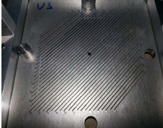
FIG. 5. Mask as machined by sinker and wire EDM at Reliable EDM. Square hole in the center allows the beam to pass through the mask, and deposit into a Faraday Cup after the FAUST array.
