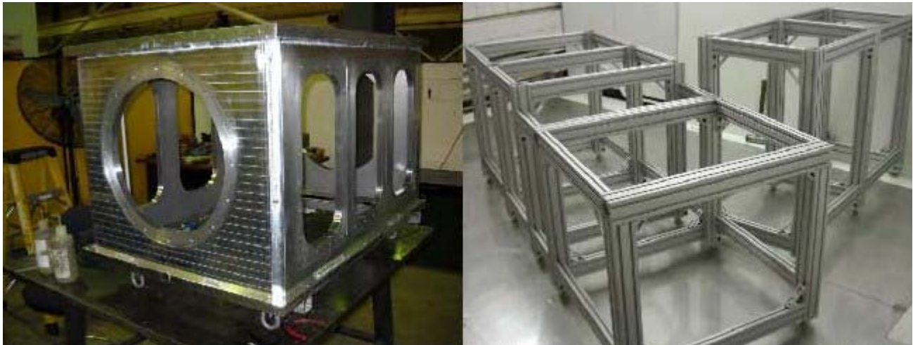
FIG. 12. Left: The vacuum box for the gas catcher is under construction and nearly finished. Right: The support stand is finished and ready for the vacuum box.
