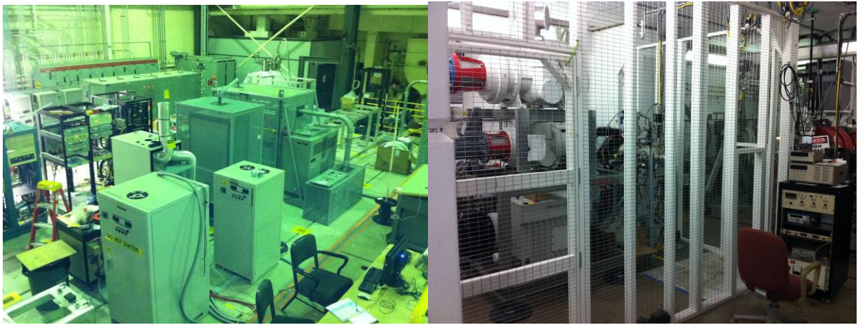
FIG. 4. Left: Equipment for the light ion guide shown positioned above the roof planks of the ion guide hall. Placement above the roof planks removes the equipment from the high radiation environment of the ion guide hall. Right: The three tier roots blower system and high voltage safety cage for the light ion guide system shown completed in the ion guide cave.
