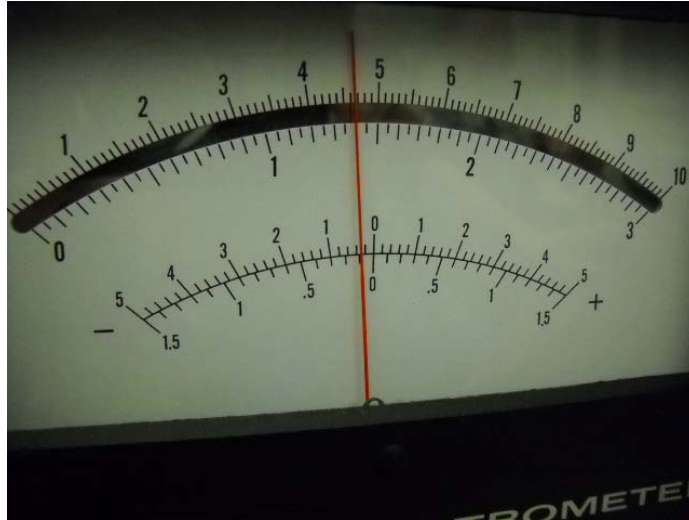
FIG. 8. Beam current of 14 \mu\text{A} of 30 MeV protons measured at the Faraday cup at the exit of the K150 cyclotron. H- ions accelerated to 30 MeV were stripped to protons at the extraction radius.
