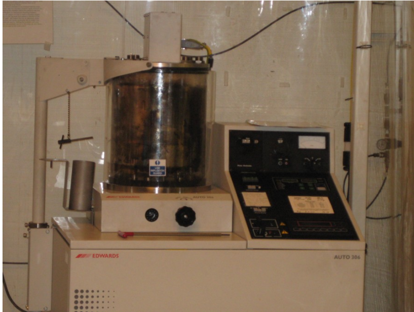
FIG. 2. Thermal evaporator at MCF.
