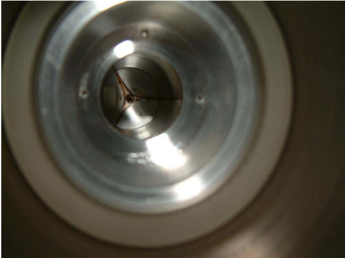
FIG. 9. The extraction plate of the CB ECR ion source after initial testing with the TWT transmitter. Note the star shape carbon coating by the hexapole field is observed.
