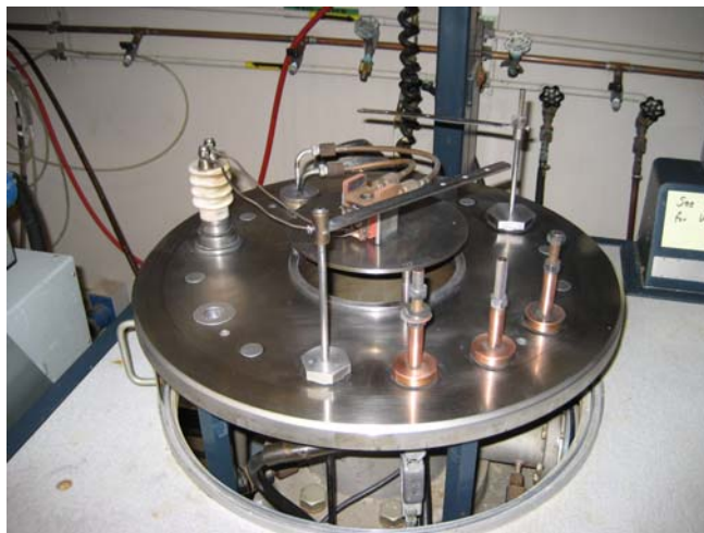
FIG. 1. Close-up of thermal and electron gun evaporator at target lab (bell jar retracted).
