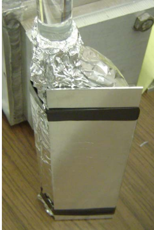
FIG. 4. Photo of Single Block Scintillator, coupled to odd-shaped and cylindrical light guides by optical cement (BC600). 1.5 mm Aluminum plate is fixed to the ion accepting side of the block scintillator.
